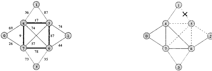
(a) A sample high-speed square-backbone network with its failure probability. Note that the number on a line indicates its failure probability \times 10^4 .
